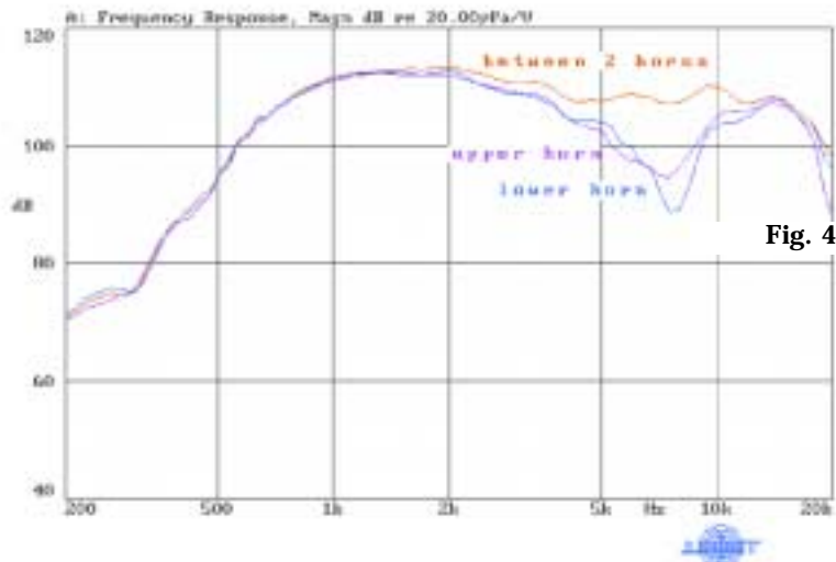
TWO HORNS VERTICALLY STACKED, 180° MEASUREMENT
